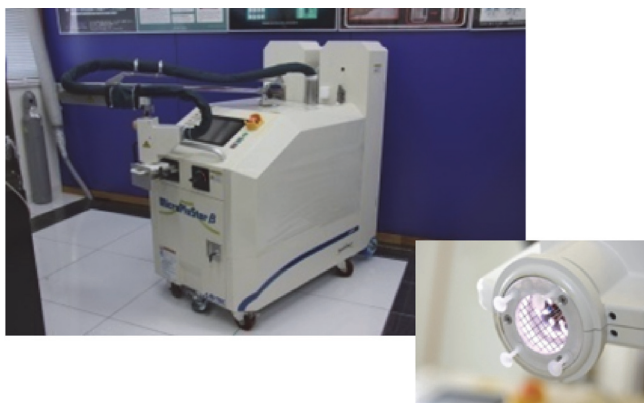
Fig. 9. Microwave plasma device, which has been used in clinical trials, so far over 3500 applications (developed together with Adtec Plasma Technology Ltd.)
