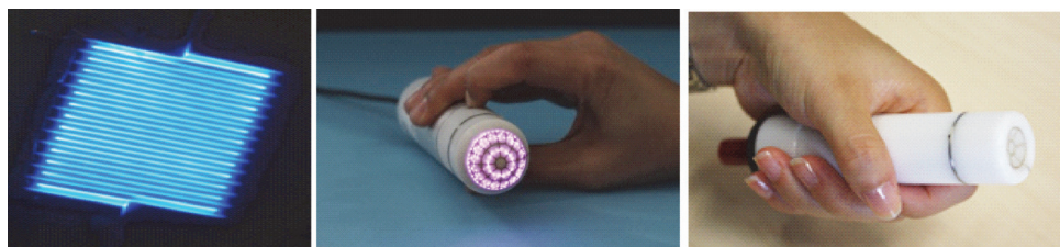
Fig. 10. Three more developments: self-sterilising surfaces (completely encapsulated work surface, which can self-sterilize with plasma – left), battery-operated design for surface treatment to remove malodour (centre), piezo (mechanically) operated plasma device (right)
